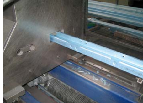
Figure 6: Wall top plate manufacture
